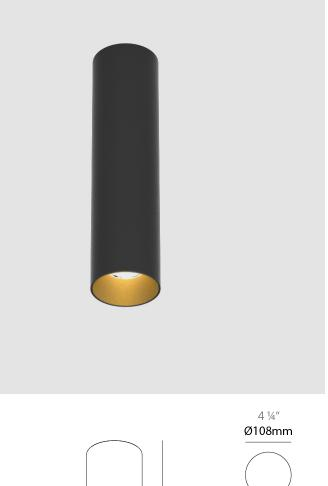
300mm 11 <sup>13/16</sup>" J-Box cover plate Included Ø 69mm 2 11/16" Ø 75mm 2 15/16"
